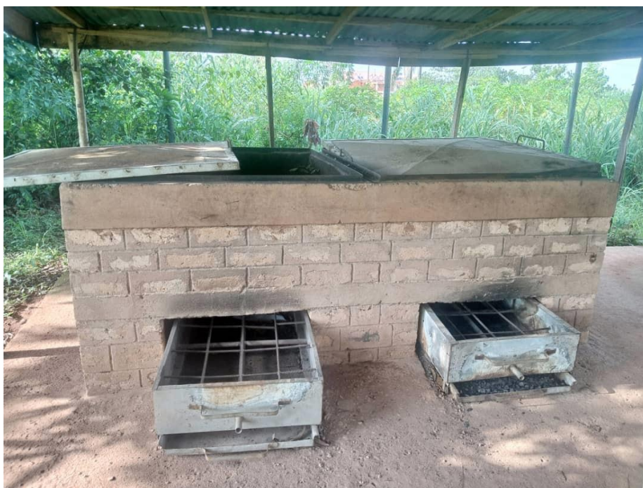
Figure 1: Fabricated smoking kiln by the Department of Fisheries and Aquaculture, PAAU
