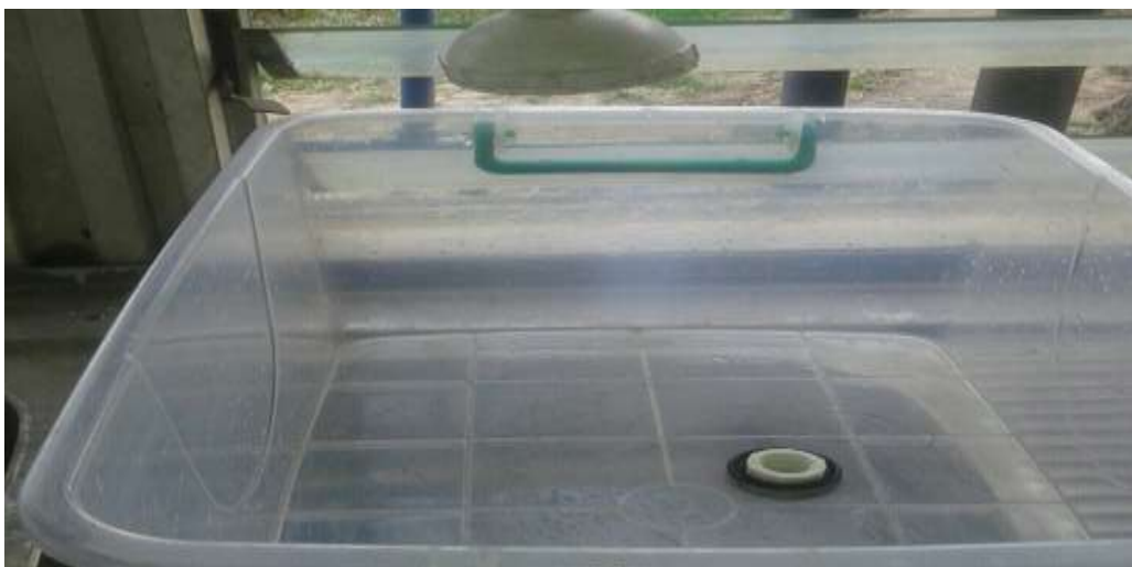
Plate 2: Constructed depuration tank with tap head for water supply.
